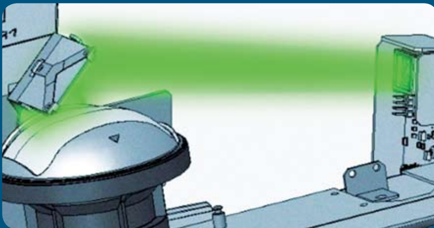
The Planar ACB mechanism works by temporarily positioning a mirror in front of the light beam coming from the lens, and then redirecting it to the Planar Color Sensor Block (CSB). The CSB measures the brightness and colors in each cube.
